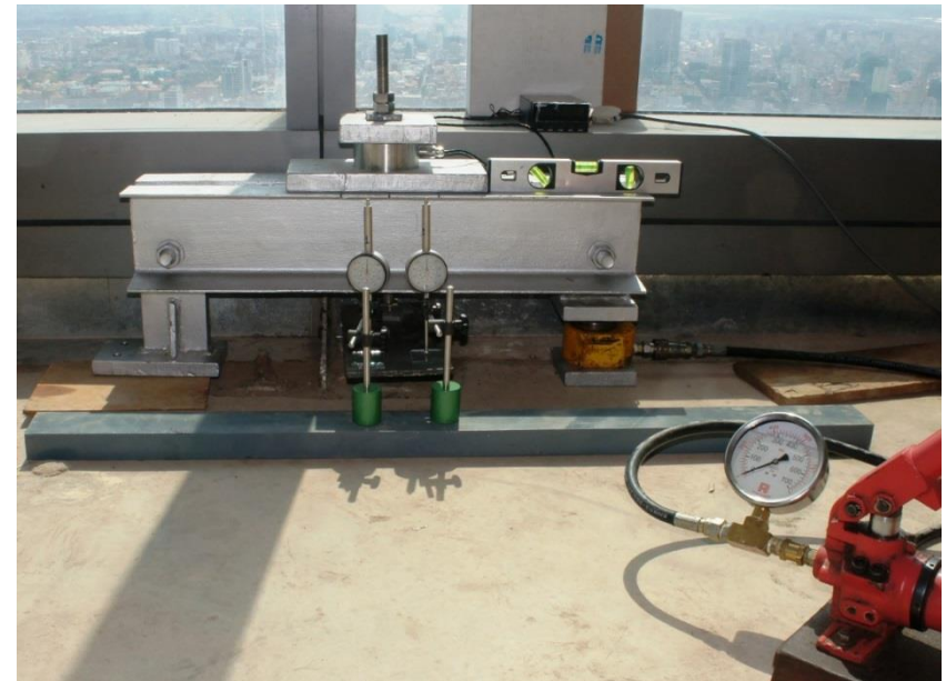
Pull-out test setup as per ASTM E488
